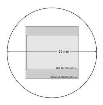
Into usable field, for example, the full-frame CCD sensor Kodak KAF 16803 sensor with 36,8x36,8 mm and a diagonal of 52.1 mm fits easily. Sensors with 45x45 mm / 64 mm diagonal can also be used.
