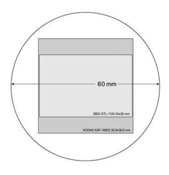
With the reducer AFFR .74x the Kodak KAF-16803 4x4 k CCD sensor with a diagonal of 52.1 mm can be used free of vignetting.
