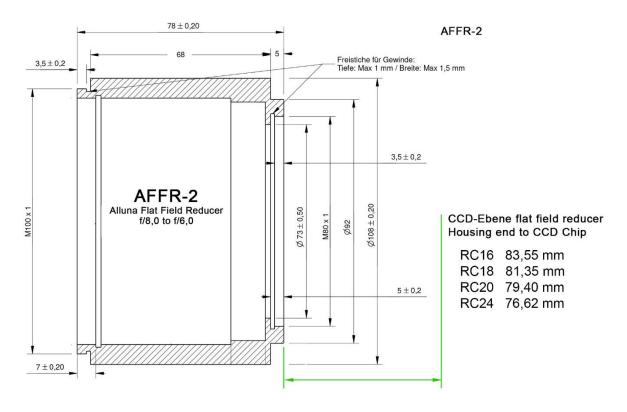
! Please note the light path of your camera, the filter wheel, as well as the filter thickness used in order to have an adapter made of the M80x1 thread connection on your camera..
