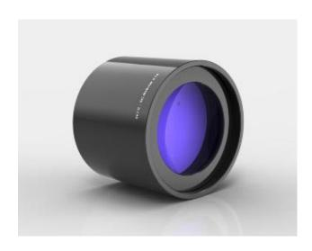
The for 4 inches for the f / 8.0 RC telescopes Alluna Flat Field Reducer x.74 (AFFR) serves two purposes. First, it corrects the image field and at the same time reduces the focal length by a factor of .74. The f/8.0 RC thus becomes an f/ 6.0 system. The picture is even, free of coma and astigmatism. The reducer can be used on all f/8.0 RC systems. To ensure a consistently high quality all corrector housing are manufactured, assembled and tested by us.
